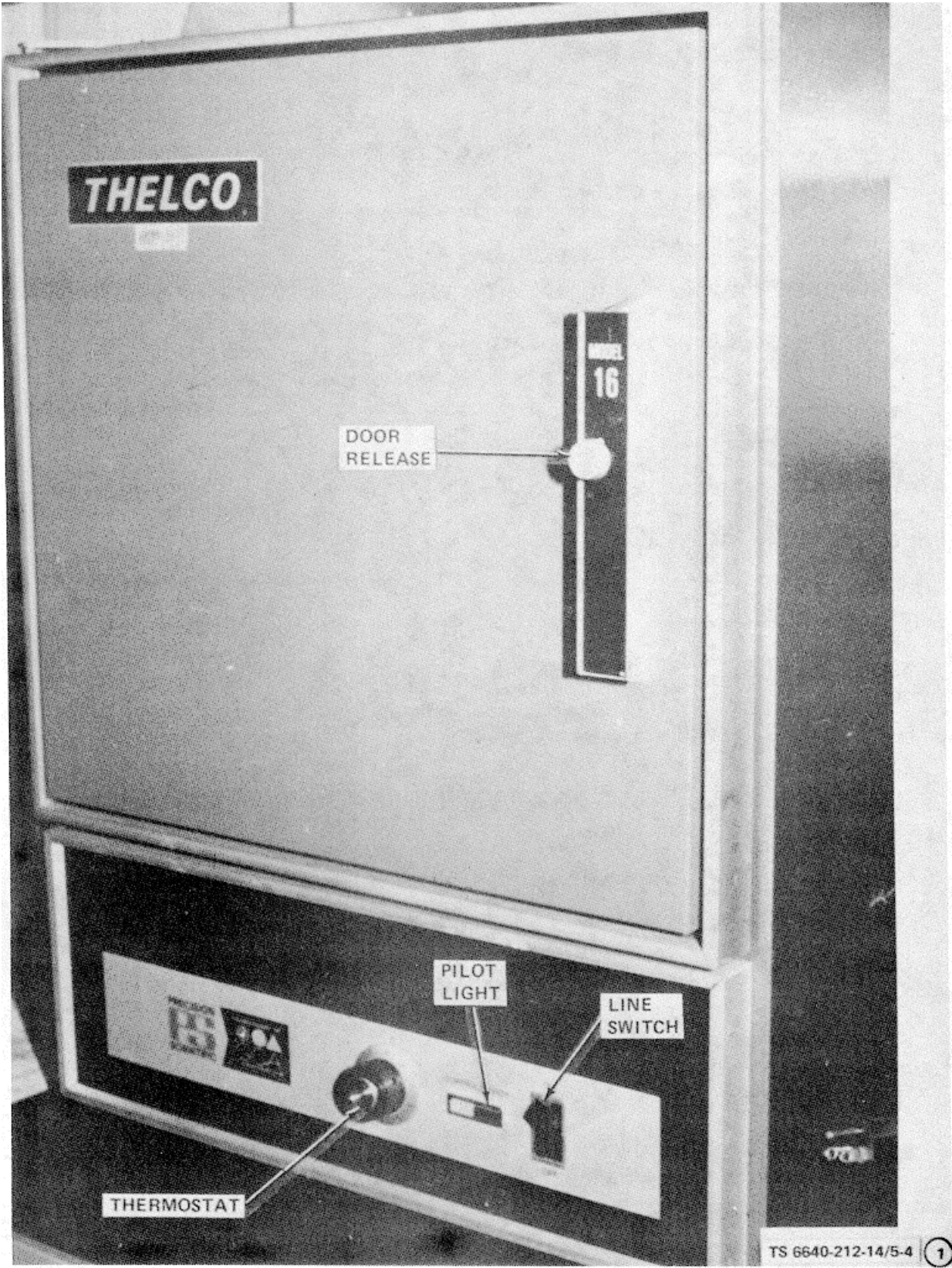
Figure 5-4. Utility Oven, Parts Location (Sheet 1 of 3)
